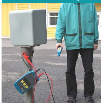
Trace electric feeding cables and other cables underground
